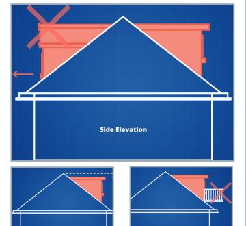
**8.** Roof extensions, apart from hip to gable ones, to be set back, as far as is practicable, at least 20cm from the original eaves. The 20cm distance is measured along the roof plane.
